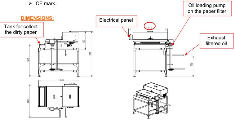
The filter shown in the drawing is relative to the model with roll of paper from 800mm, for the model with 600 mm paper roll, remove 200mm to the red circled measure -200mm.
