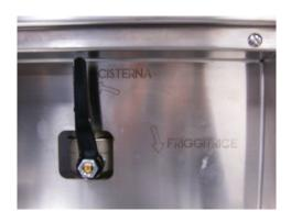
It is possible to decide whether to send the filtered oil to the fryer's tank or to the oil recovery tank (see image).
