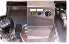
Loading of the oil into the fryer automatically (controlled by MAX and MIN levels) or manual. If the oil level exceeds the set one, the overfull drains the excess oil into the recovery tank. Maintaining a certain temperature through one resistance in the oil recovery tank so that the oil doesn't solidify.
