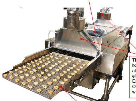
There are two aspirators in the boiler, one at the inlet and one at the outlet, in order to eliminate the vapor generated. Each aspirator has an outlet of Ø120 mm, to be connected with a suitable system.
