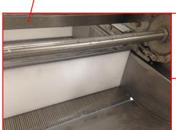
The product is transported along the entire cooking path by means of special Teflon pallets.
