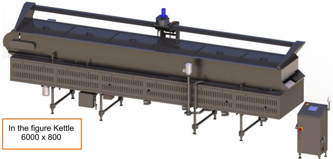
The industrial paddle kettle has been designed for the continuous boiling of products such as pasta (the most varied types), spaghetti, rice, gnocchi, tortellini, ravioli etc ... It is available in various sizes and versions depending on the production required and the type of power supply: gas or electric.
