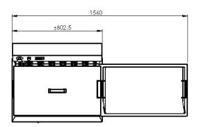
Equal overall dimensions for both 13.5 kW version and 22.5 kW version.
